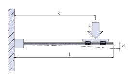
The deflection of a Slide beam acting as a cantilever and using a Long Flange Clamp (as shown opposite), will be a maximum at the free end when the load is at the outermost extremity of its stroke. This maximum deflection is given by the following equation:
