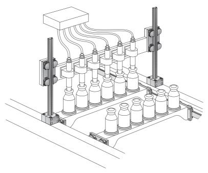
**SL2 System** is used for vertical and horizontal guidance on a bottle filling machine in the cosmetics industry.
