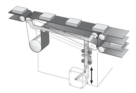
**SL2 System** is used as the vertical guidance in a food industry application to move a diverting conveyor between two further conveyors alternately. High speed and high duty operation driven by a crank arm.
